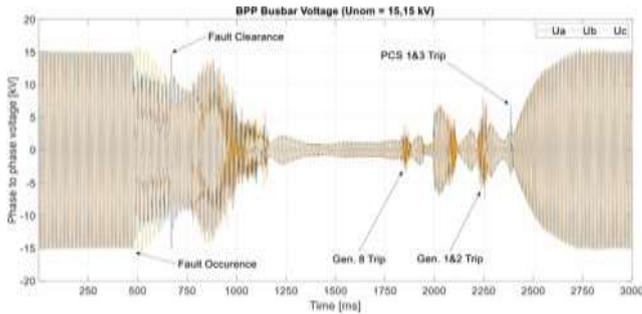
Fig. 2 Ph-Ph three-phase voltages at the medium voltage busbar during and after the event (Source: Graciolica)
