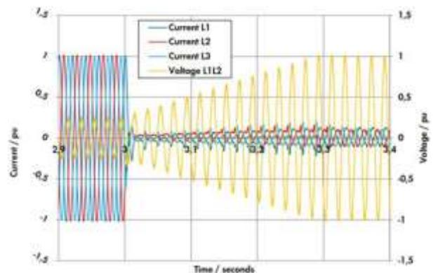
Fig. 6 Voltage recovery due to the SW protection after clearance of the SC, per the firmware installed currently at this site (Source: PCS Manufacturer, SMA)
