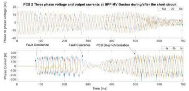
Fig. 4 PCS 2 measurements during and after fault (top) PCS 2 AC output voltage, (bottom) PCS 2 AC output current
