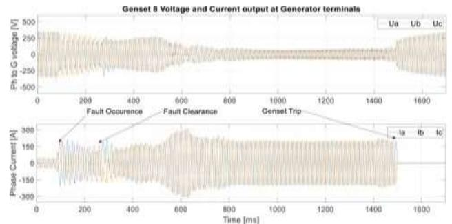
Fig. 5 Genset 8 output measurements after fault occurrence (top) Genset 8 output voltage, (bottom) Genset 8 output current (Source: Graciolica)
