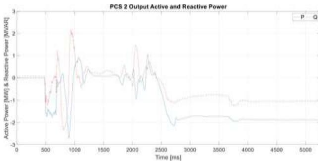
Fig. 3 PCS 2 active and reactive power output during and after the event until stabilisation (Source: Graciolica)
